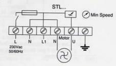
L1 : Live supply bypassing the Fuse & On/Off switch (which is on the side) or it can be used as a supply for 3 wire motors.
