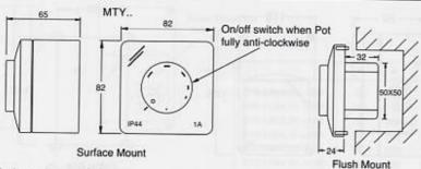
Electrical entry is possible from the bottom or from the back.
